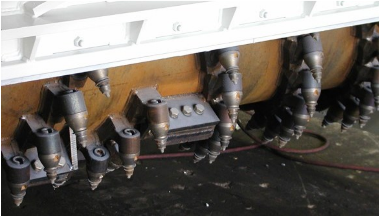
Figure 1-2 Teeth on rotating drum of milling machine [31]
