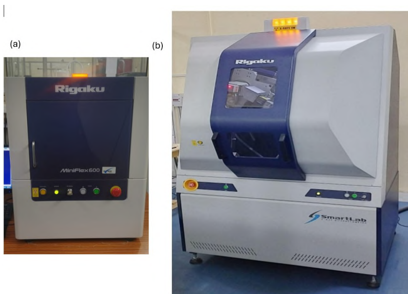
Fig. 2.3 (a) Bench-top XRD and (b) HR-XRD used for diffraction measurements.
