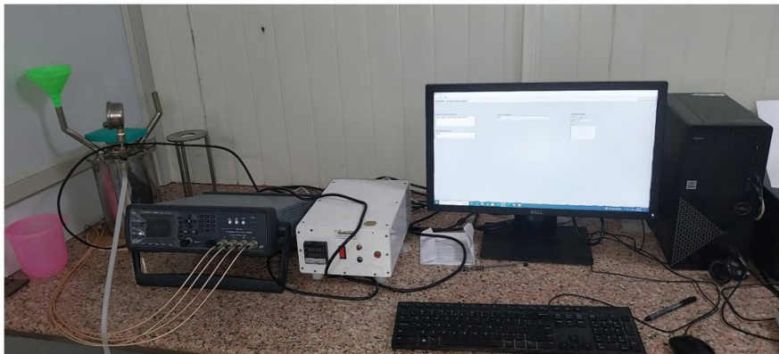
Fig. 2.6 Keysight LCR meter used for dielectric measurements.
