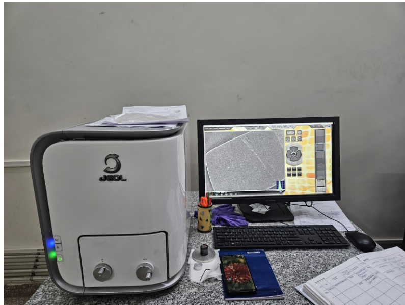
Fig. 2.5 BT-SEM used for microstructural analysis.
