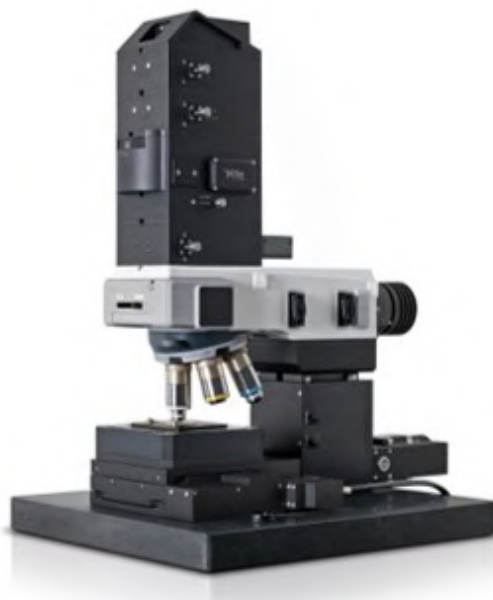
Fig. 2.9 Raman Instrument used for room temperature measurements.
