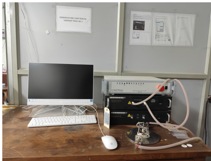
Fig. 2.8 Polarization vs. electric field (P-E) loop tracer by Radiant technologies.
