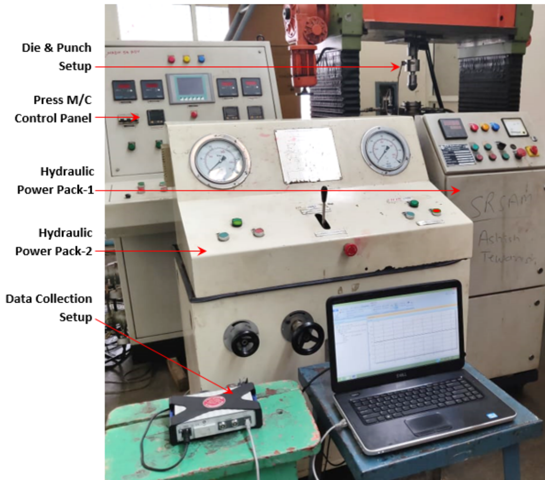
Figure 3.21: Rubber assisted sheet Hydro-forming Set Up
