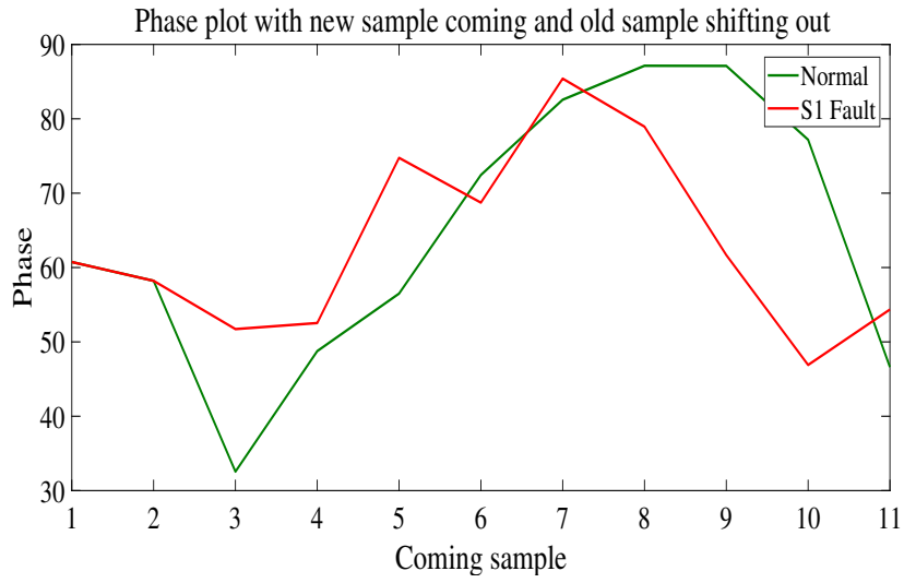
Figure 5.17: Phase of WFCs of window of 11 samples of voltage signal under fault condition at S_1 .
