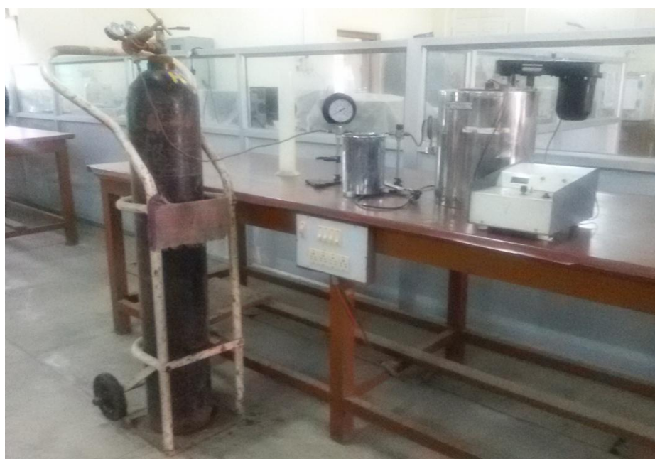
Figure 4.10 Schematic view of Calorimeter
