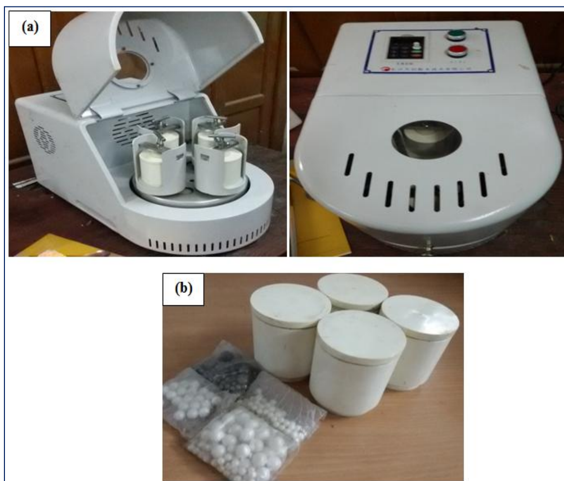
Figure 4.6 (a) Planetary ball mill, (b) Jar and grinding balls ( ZrO_2 )
