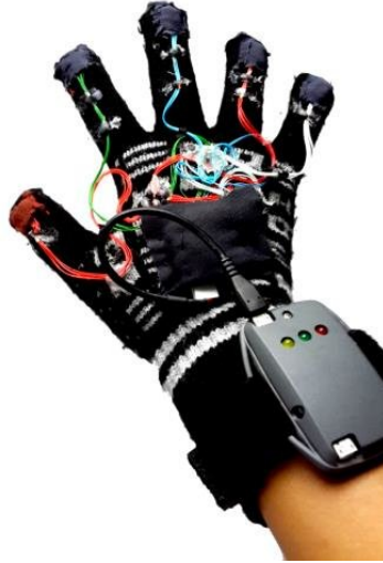
Figure 2.1: A type of data glove used for capturing hand joint motion.
