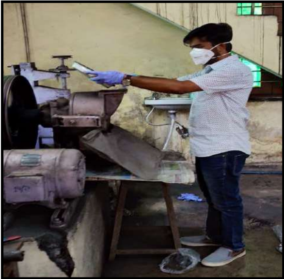
Fig. 4.19: Photograph of pulverisation of coal samples
