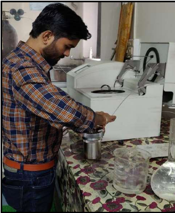
Fig. 4.21: Photograph of operating Bomb calorimeter
