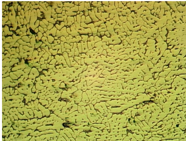
Figure 4.34: Optical micrograph (b) 140A_21V at Gas flow rate: 14LPM and Heat Input of (b) 9.4kJ/cm
