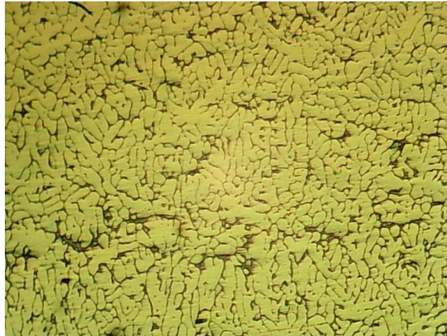
Figure 4.13: Optical micrograph(c) 180A_15V at Gas flow rate: 10 LPM and Heat Input of (c) 8.6kJ/cm
