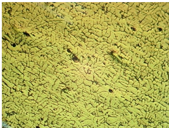
Figure 4.39: Optical micrograph (c) 180A_15V at Gas flow rate: 18LPM and Heat Input of (c) 8.6kJ/cm
