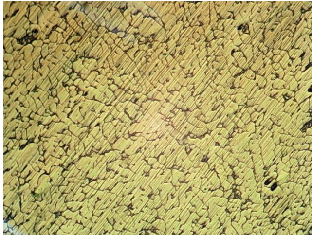
Figure 4.17: Optical micrograph (c) 180A_15V at Gas flow rate:14 LPM and Heat Input of (c)8.6kJ/cm
