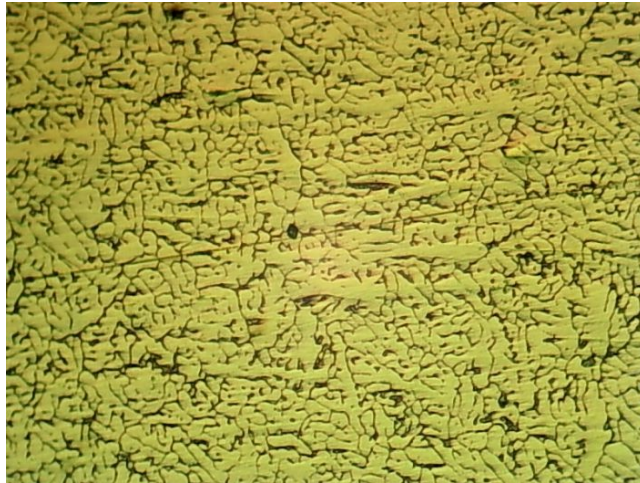
Figure 4.30: Optical micrograph (b) 140A_21V at Gas flow rate: 10LPM and Heat Input of (b) 9.4kJ/cm
