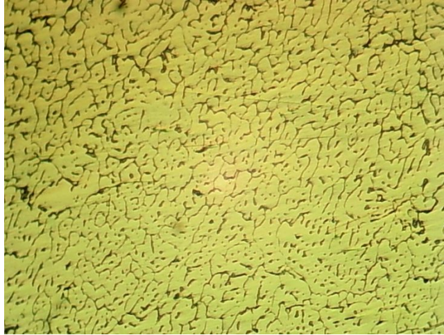
Figure 4.11: Optical micrograph (a) 140A_15V at Gas flow rate: 10LPM and Heat Input of (a) 6.7kJ/cm
