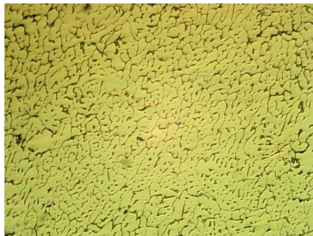
Figure 4.10: Optical micrograph of MIG welded A6061 alloy: Fusion Zone (FZ) For Gas flow rate of 10LPM and different heat input the microstructural changes can be seen in Fig. 4.11(a), 4.12(b), 4.13(c) and 4.14(d). Welding Heat Inputs for in Fig. 4.11(a),
