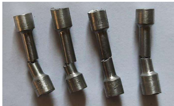
Figure 5.15: Fracture pattern of the tensile test sample of A319 alloy
