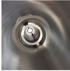
Fig. 11. Photograph of a precision-machined biperiodic MTM SWS studied in hot tests.
