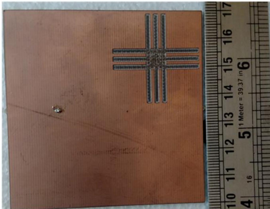
Figure 5.5 A fabricated prototype of the single meandered-cross shaped slot antenna
