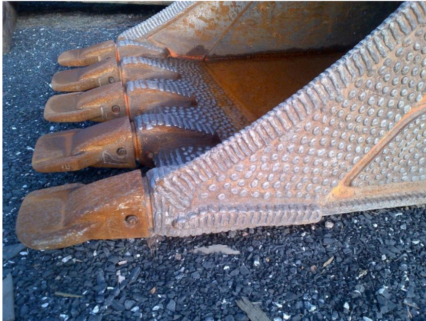
Figure 1-1 Hard facing edges of the bucket to prevent excessive wear [1]
