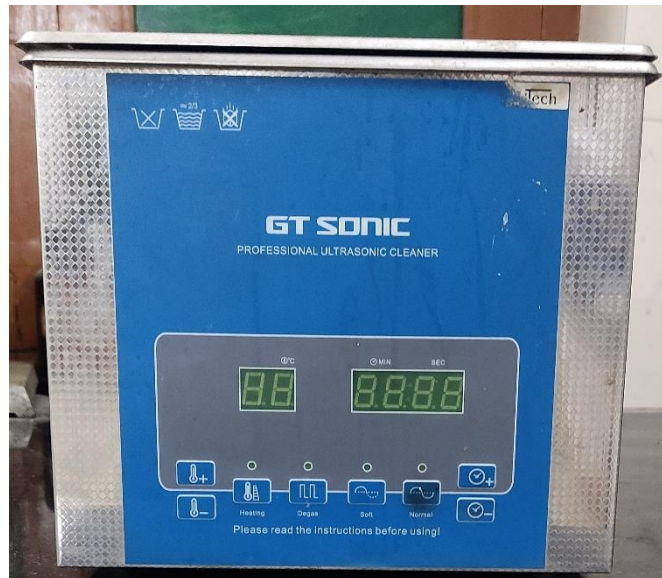
Fig. 3.3. Photograph of bath sonicator (Model: GT-1730QTS, Frequency: 33/40 kHz, Power: 100 W).
