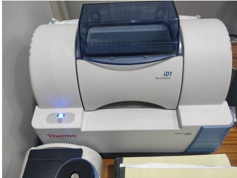
Figure 3-4. Fourier Transformed Infrared test setup
