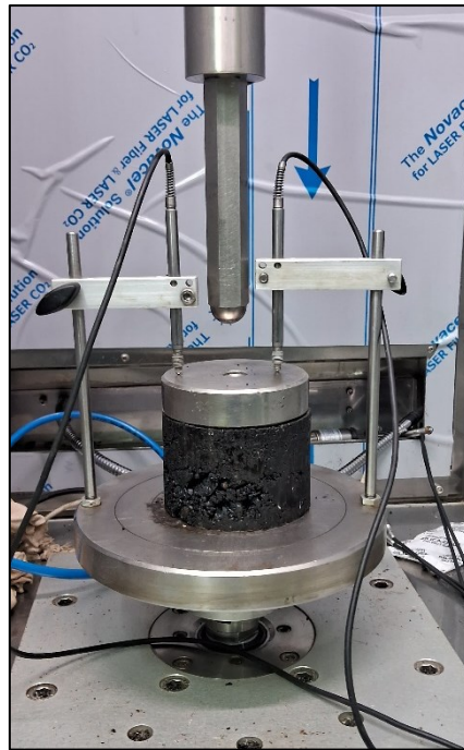
Figure 3-5 Dynamic creep compression test
