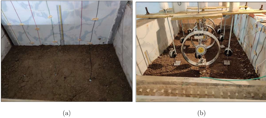
Figure 3.9: Rectangular EK model image (a) Soil chamber installed with dummy electrode (b) Soil chamber with dial gauge and proving ring
