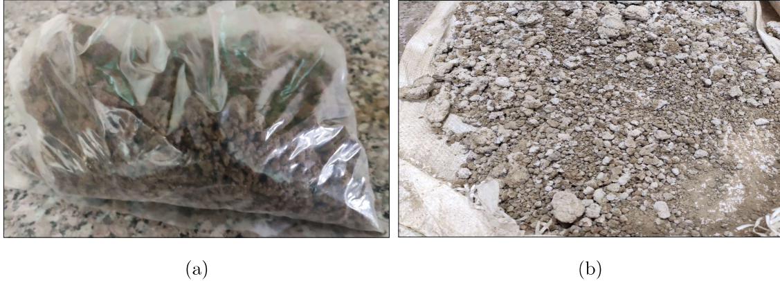
Figure 3.6: Interaction of alkali solution with soil (a) polythene bag (b) air drying of alkali interacted soil
