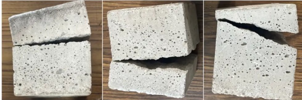
Figure 4.18 Spalled mortar cubes (MK10, NS3, MK10NS3)
