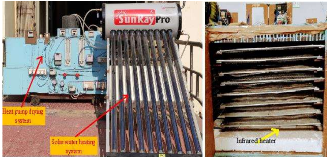
Fig. 5.2: Photograph of the developed experimental setup of SIAHPD and drying chamber interior
