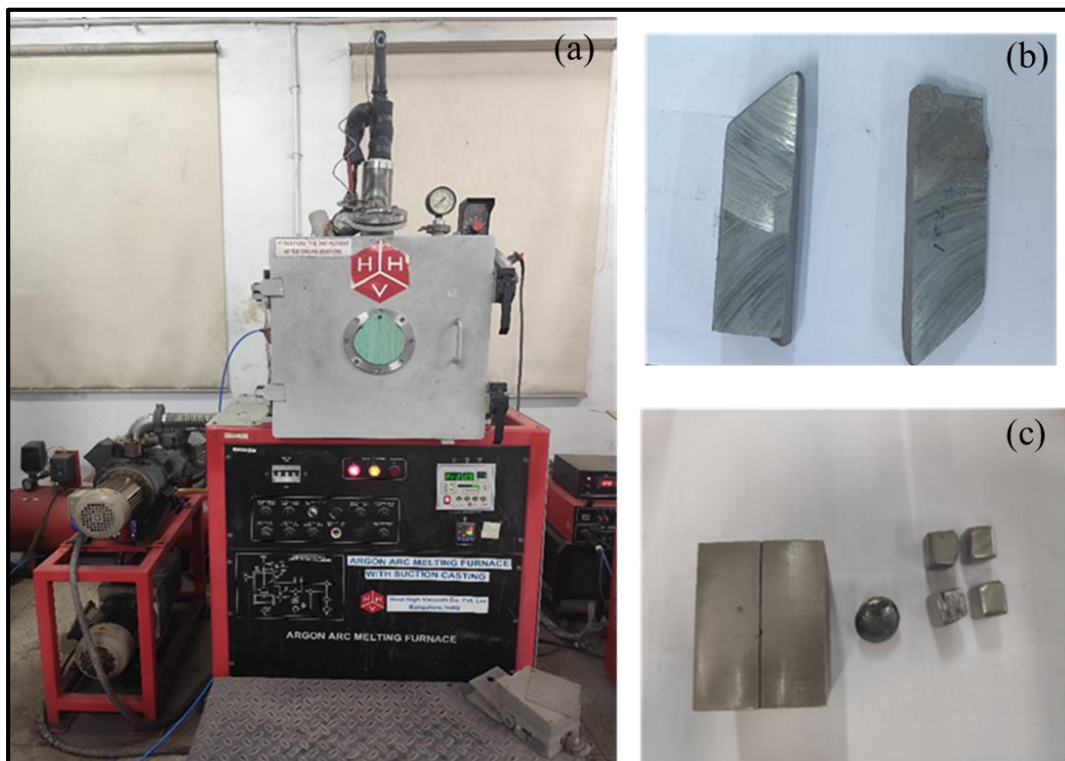
Figure 3.1- (a) Vacuum Arc Melting facility for Ingot preparation and (b)-(c) prepared master alloy ingots.
