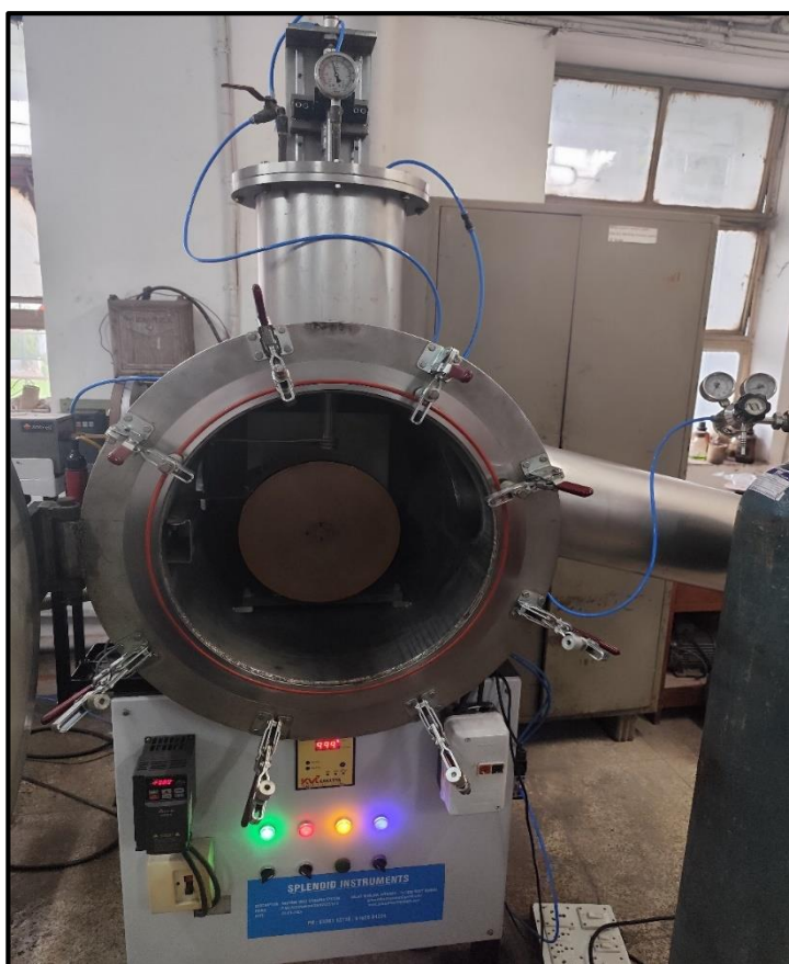
Figure 3.2- Melt spinning facility for preparation of Amorphous Electrical Steel.
