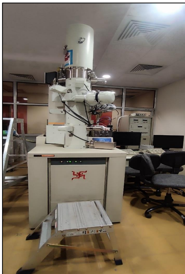
Figure 3.8- Transmission electron Microscopy facility for material characterisation.
