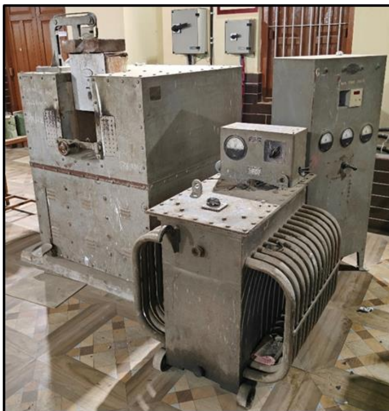
Figure 2.8: Resistance Furnace used for hardening of dry MMO pellets
