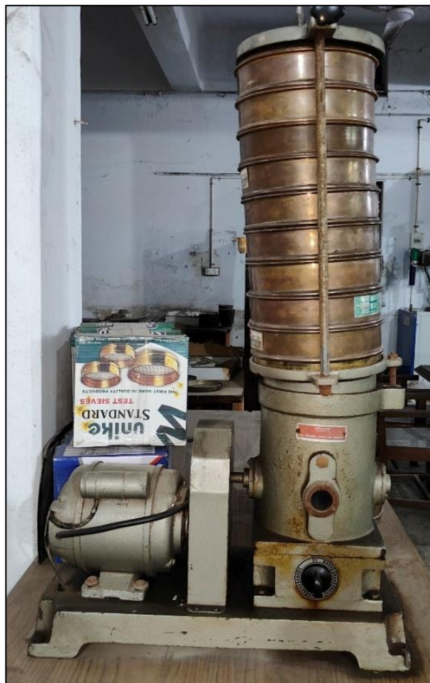
Figure 2.5: Setup used for sieve analysis of multimetallic magnetite ore fines
