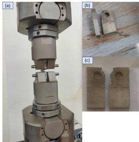
Fig. 2.21 (a) Grip for fracture test, (b) and (c) are the fractured CT sample by J1c process.
