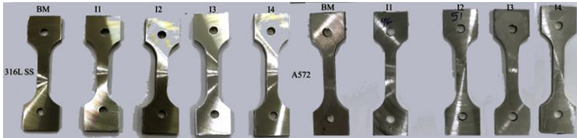
Figure 3.8: Base and Welded Tensile test specimens of 316L SS and A572 gr. 50
