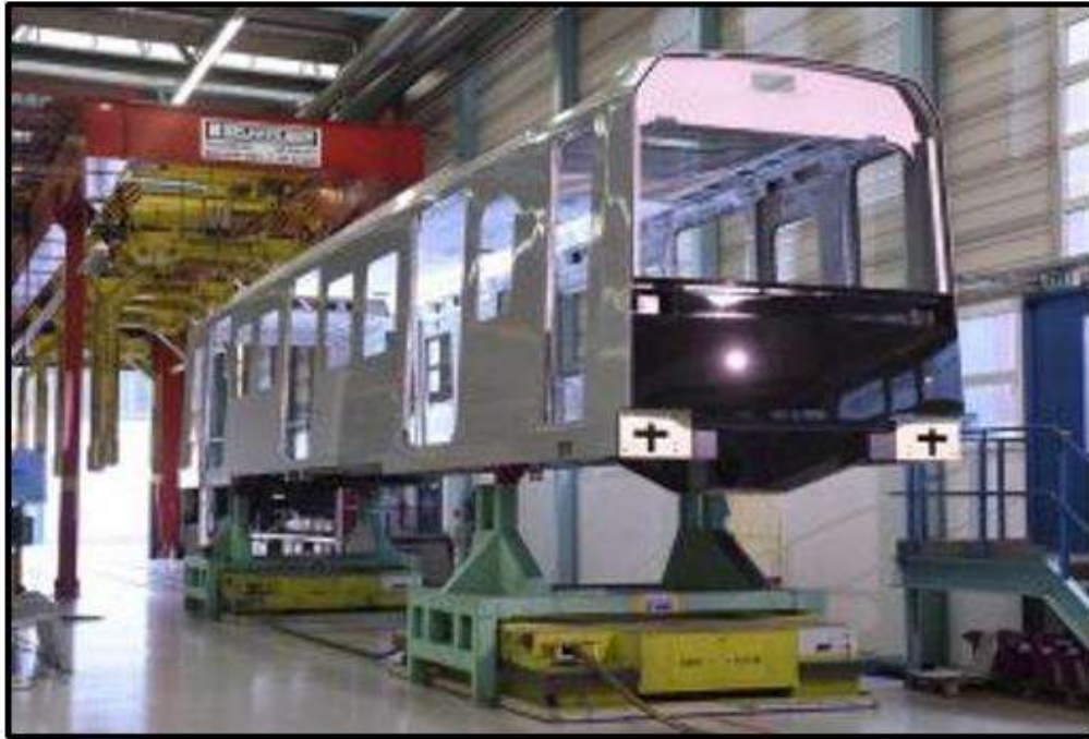
Figure 1.2: Typical car-body of high-speed train made of aluminium alloy [3]
