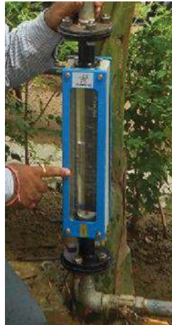
Figure- 6.3 Rotameter for Measuring of Discharge
