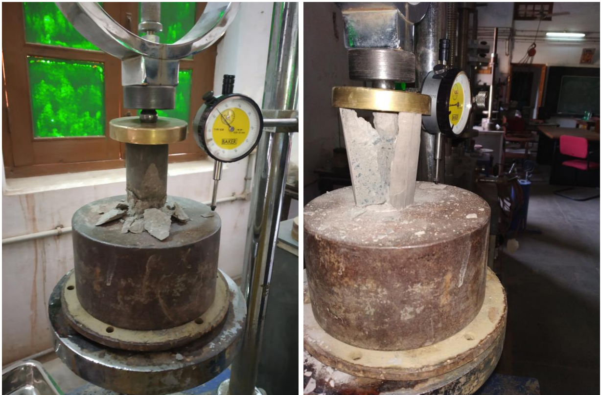
Fig: 4.6 UCS Testing of Pond ash-GGBFS Mixes
