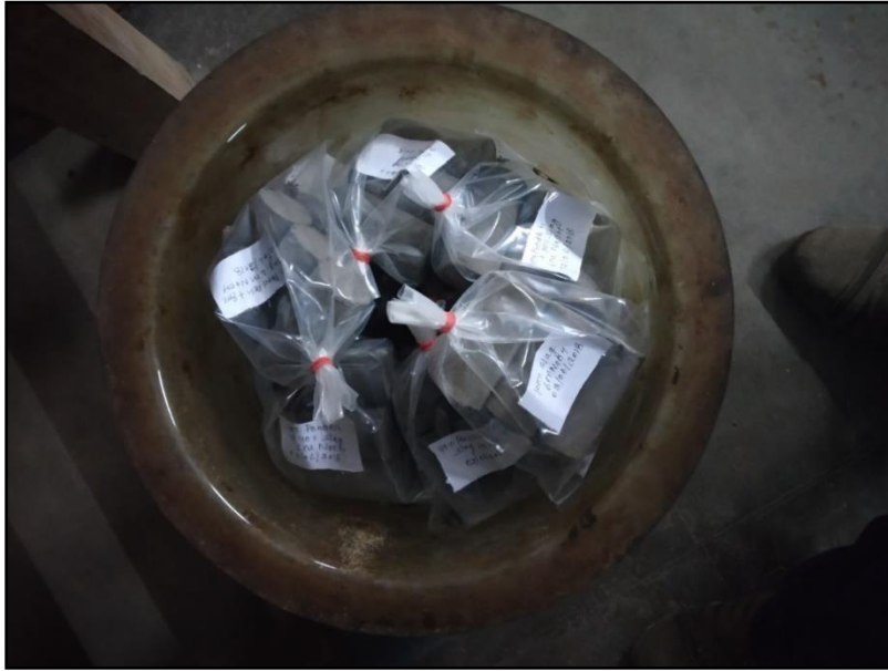
Fig: 4.5 Polythene curing of Pond ash-GGBFS Mixes for different curing period
