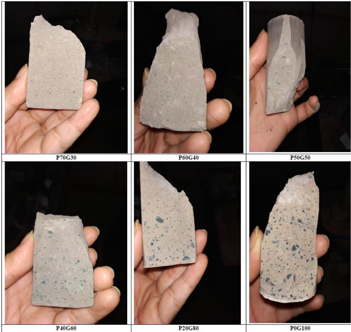
Fig: 4.20 Image of Pond Ash-GGBFS broken samples during UCS analysis
