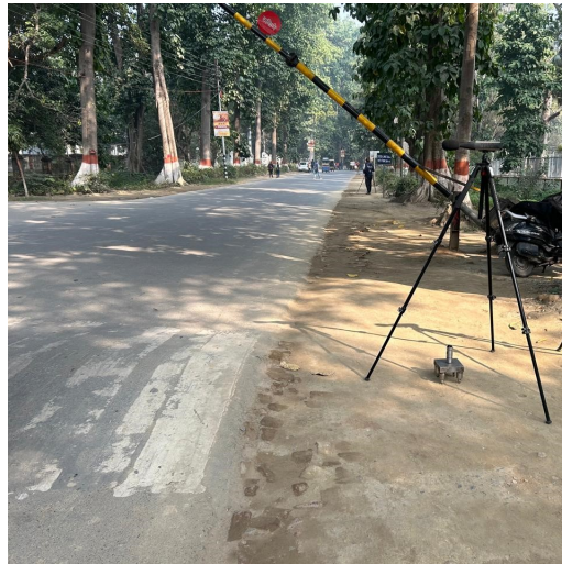
Fig. 4.16 Illustrative layout of a speed hump profile and the associated sensor deployment.
