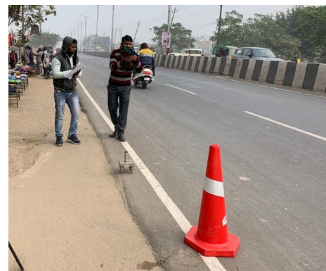
(b) Manual LIDAR speed measurement and vehicle annotation
