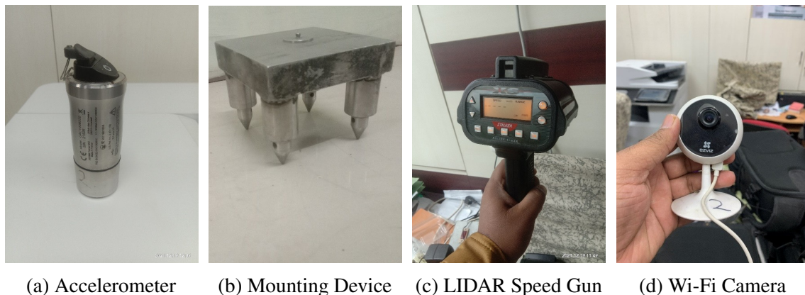
Fig. 4.1 Instrumentation used for vehicle-induced vibration acquisition.
