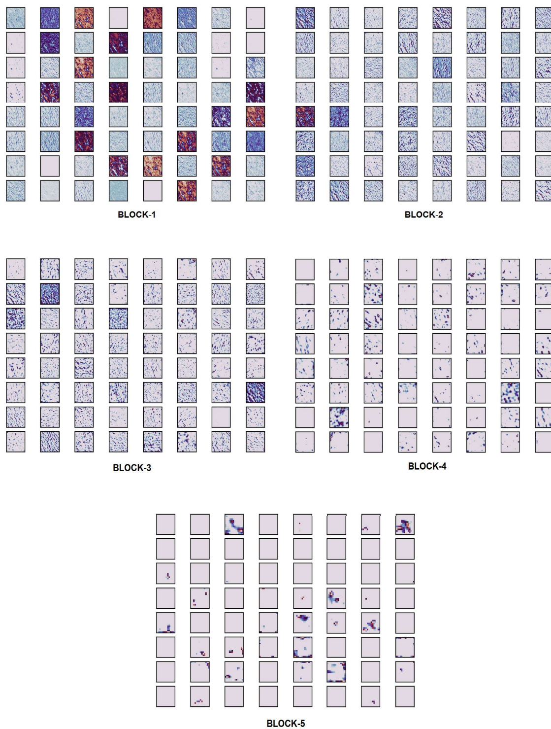
Figure 4.8: Visualization of the feature maps of one of the images extracted from Block-1 to Block-5 in the VGGNet-16 Model.
