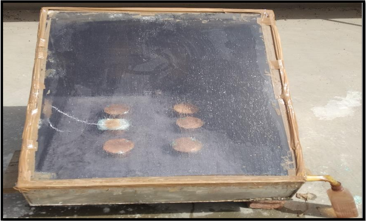
Fig. 3.2 Pictorial view of the experimental setup for solar still coupled with PCM stored in copper cylinder
