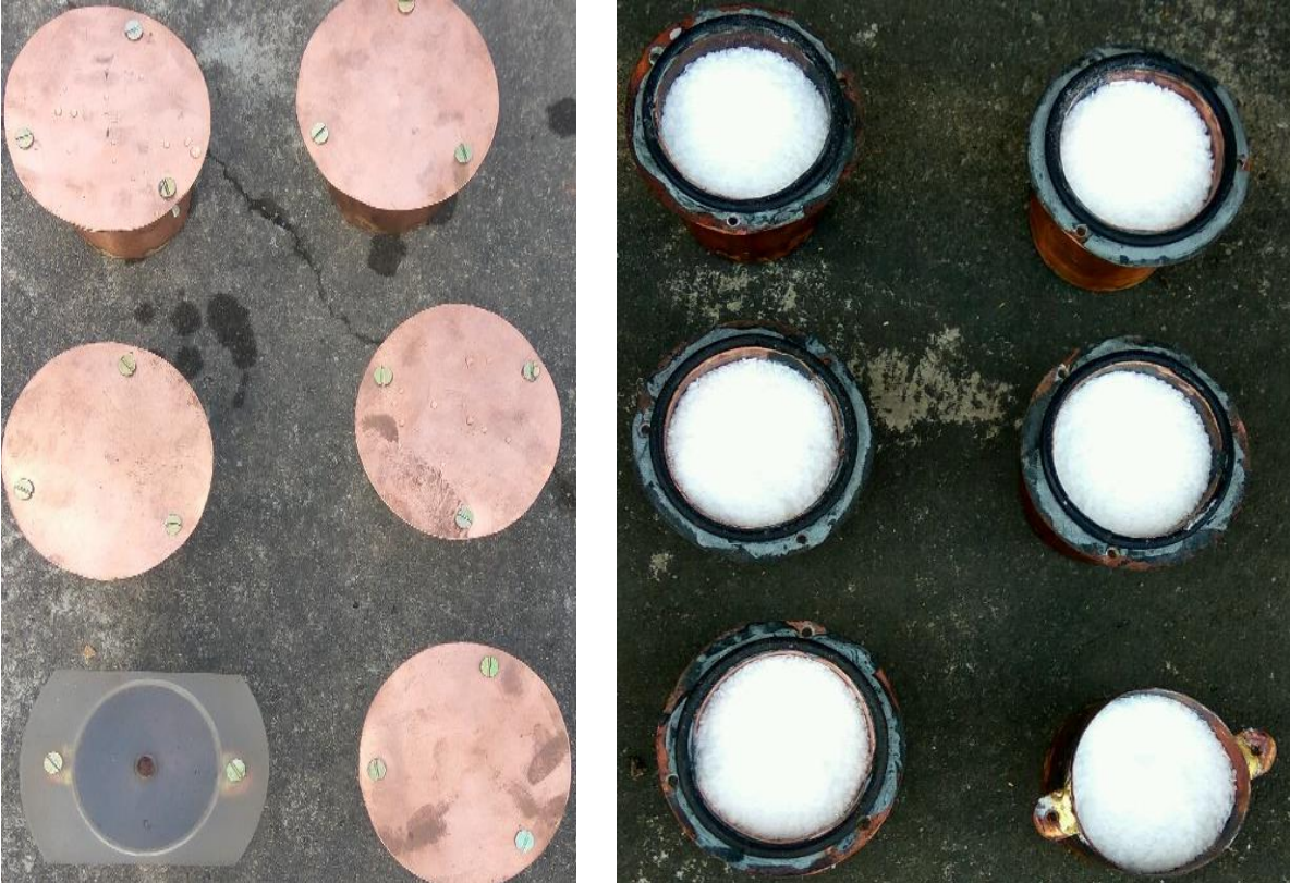
Fig. 3.3 Pictorial view of PCM loaded copper cylinders
