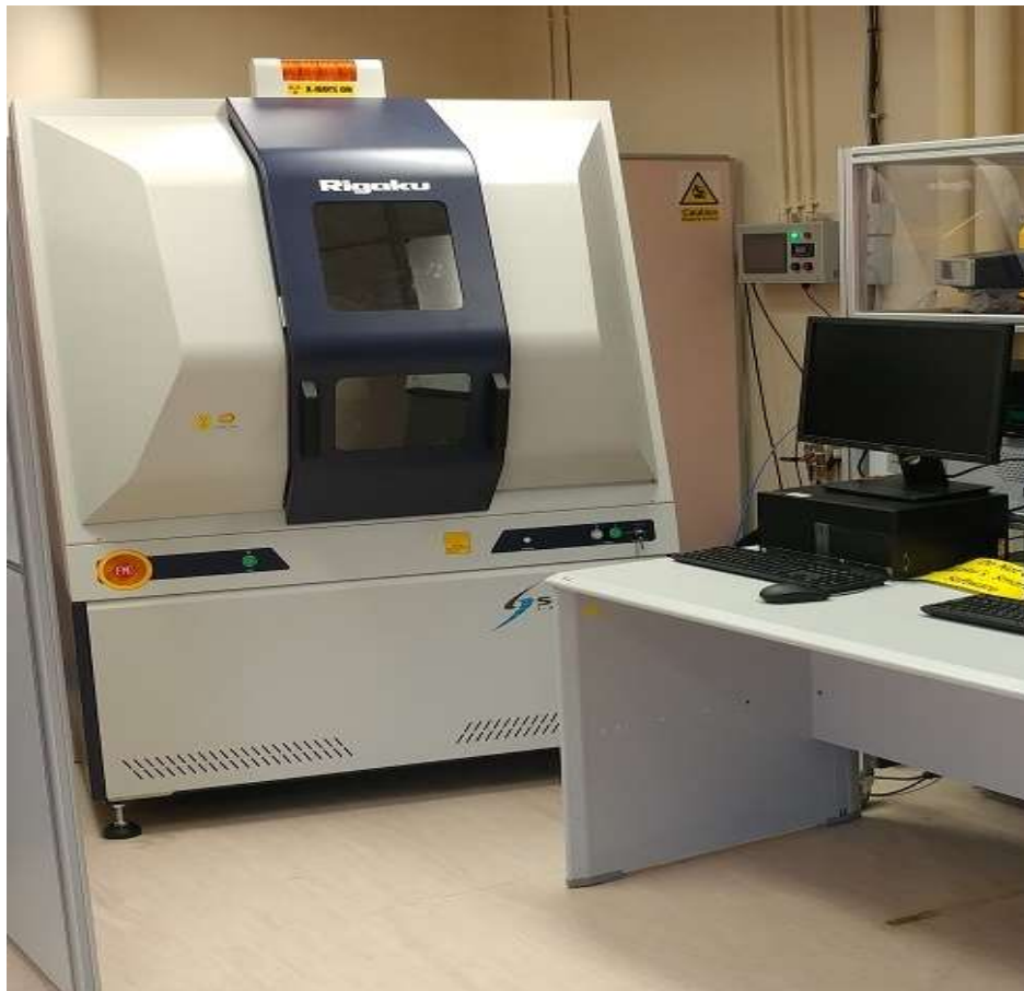
Figure 2.13 X-Ray Diffractometer Instrument.
