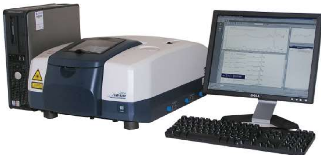
Figure 2.14 FTIR Spectrometer Instrument.
