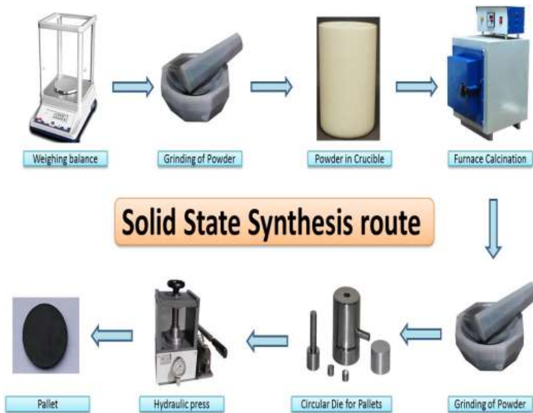
Figure 2.4 Schematic diagram for preparation of pellets through Solid-State Synthesis route.
