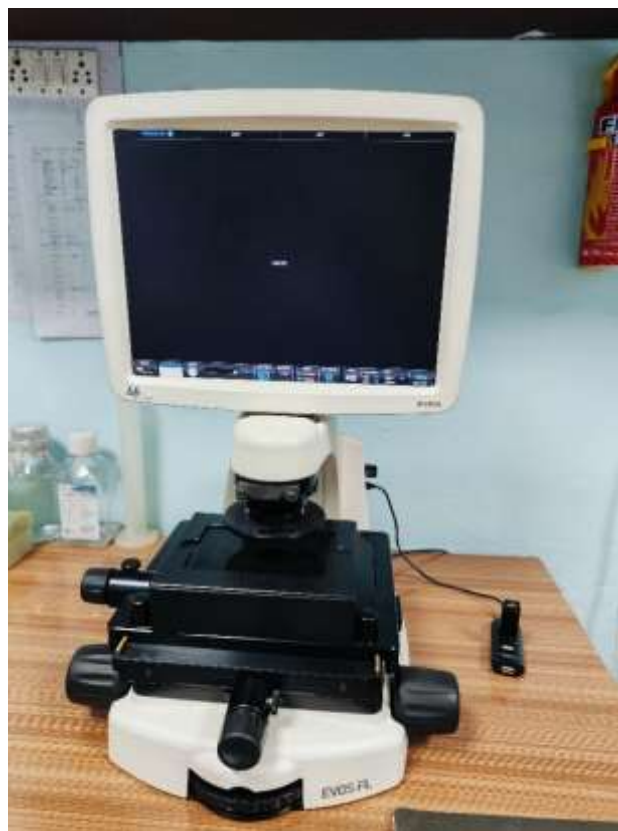
Figure 2.20 Inverted fluorescence phase contrast microscope.
