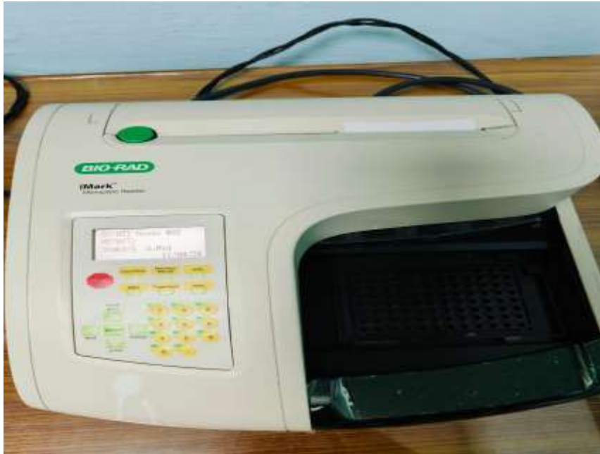
Figure 2.19 Bio-rad iMark™ microplate absorbance reader for cellular analysis.
