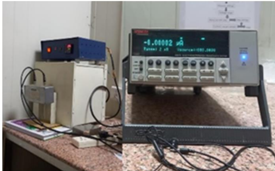
Figure 2.22 Pyroelectric measurement system (Keithely 6517B electrometer).
