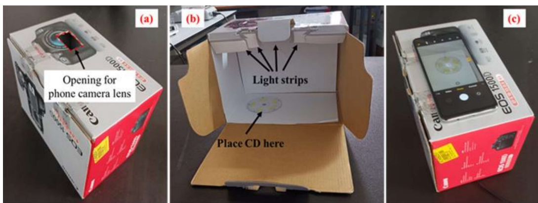
Fig. 5.4 Lightbox setup for image capture: (a) An opening is created in the top surface of the box to accommodate the smartphone camera lens; (b) Four LED light strips covered with paper are secured on the top surface with the help of double-sided tape, and after the development of the color, the CD is placed inside the light box at indicated placed; (c) All sides of the lightbox are closed with the lights on. The phone camera lens is placed over the opening, and the image is captured for analysis.
