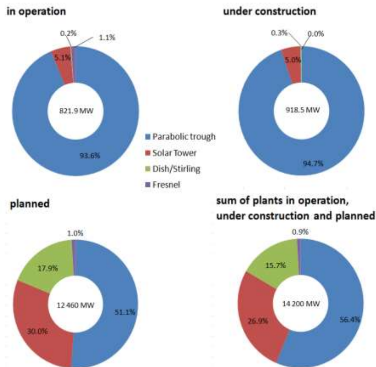
Figure 2.5: Contribution of different solar concentrating technologies for power generation [100]
