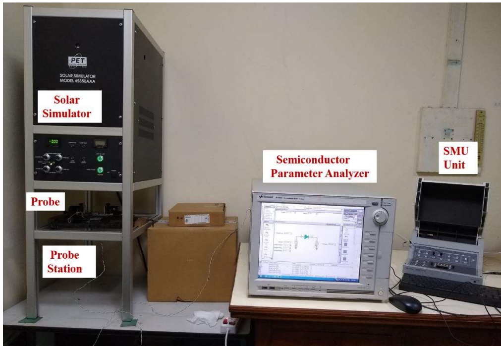
Figure 1.15: Experimental measurement setup for the electrical characterizations.
