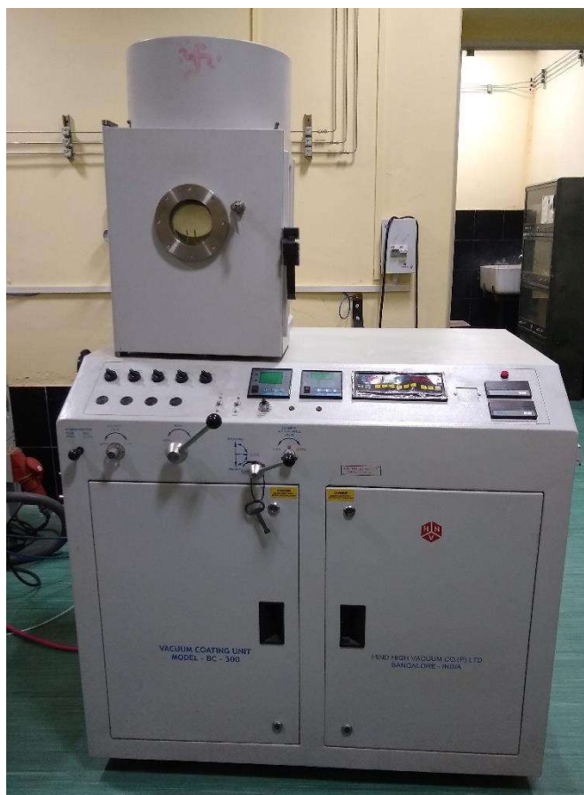
Figure 1.9: Thermal evaporation deposition instrument for metal electrode deposition.
