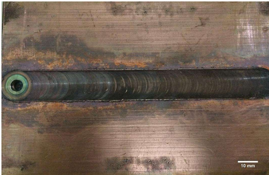
Figure 6. 1 The surface appearance of FSPed Cu/ZrO 2 surface composite
