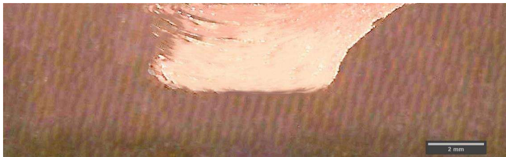
Figure 6. 2 The cross-sectional macrostructure of FSPed Cu/Zirconia surface composite
