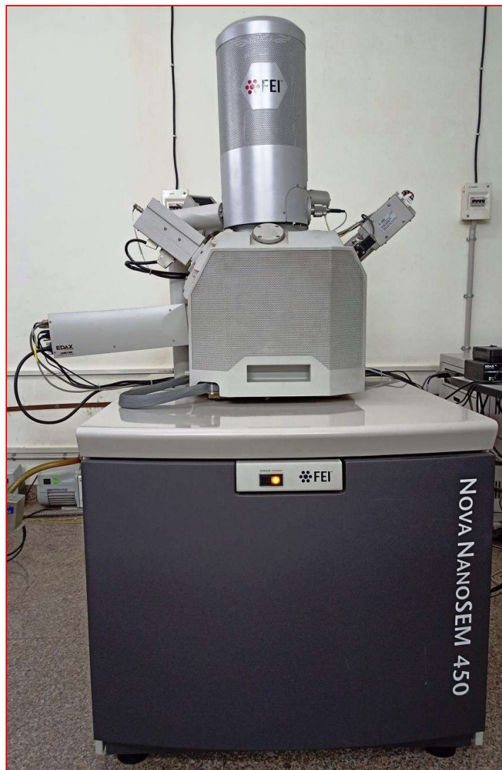
Figure 2.3 FE-SEM instrument (model: Nano Nova SEM 450).
