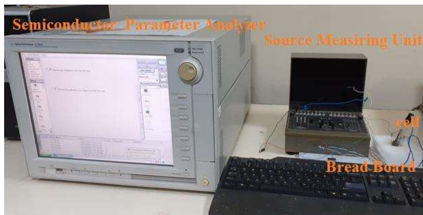
Figure 1.11: Semiconductor parameter analyzer for the measurement of various electrical parameter
