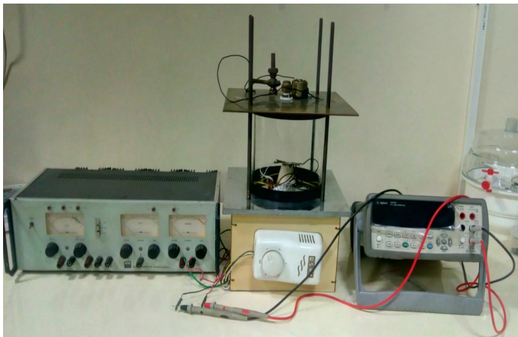
Figure 3.9: Front view of In-house developed a gas-sensing measurement system.
