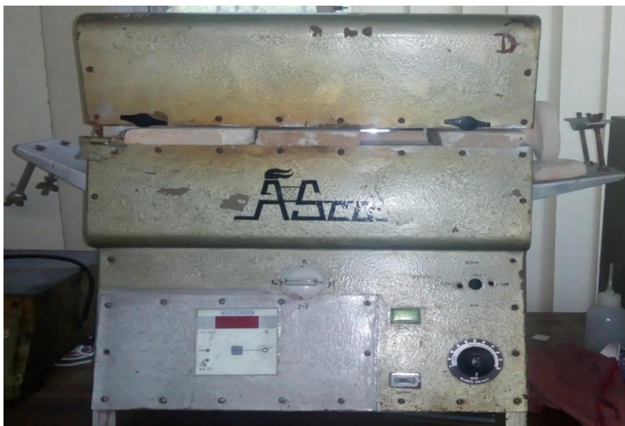
Figure 3.4: Front view of a calcination furnace
