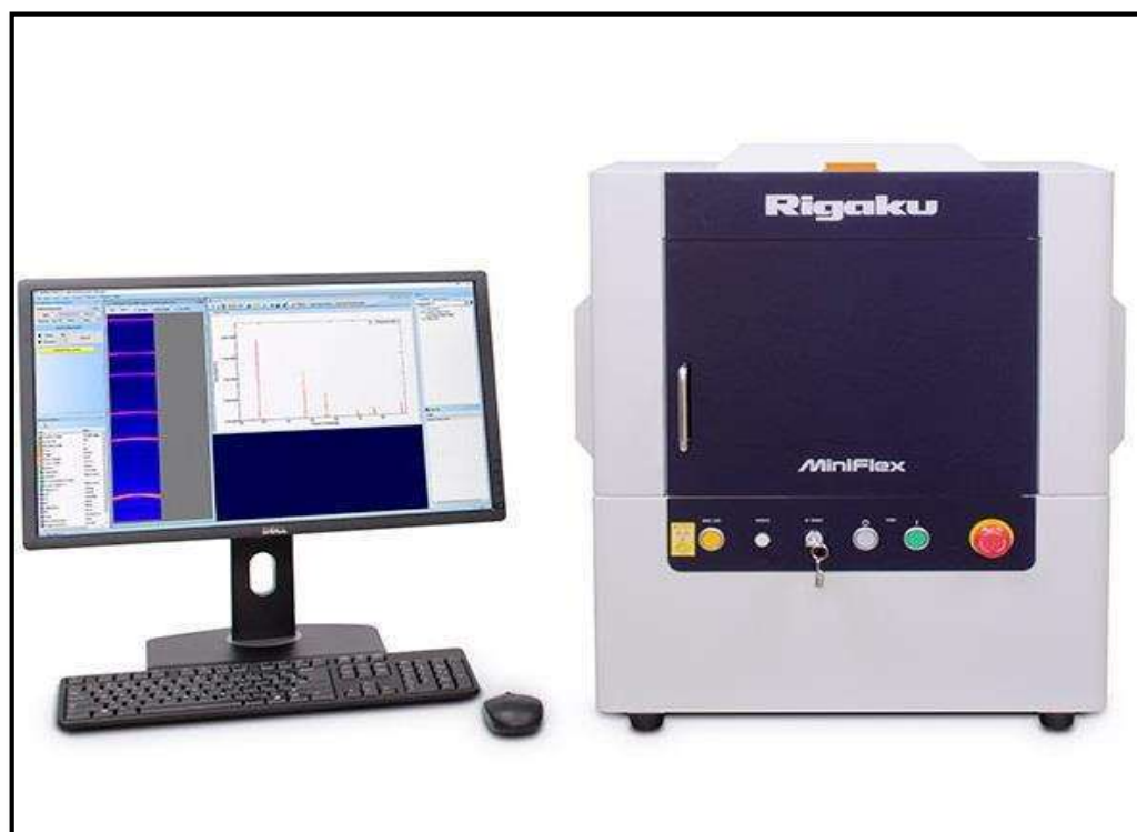
Fig.2.2. Powder X-ray diffractometer, Rigaku Miniflex600 (Japan).
