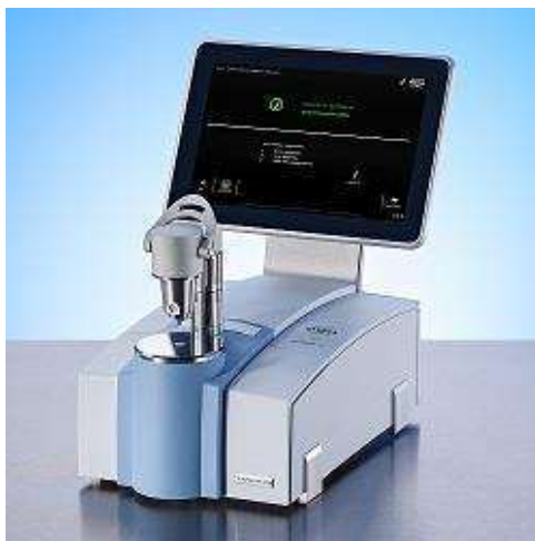
Fig.2.3. FT-IR Spectroscopy (Bruker, ALPHA model)
