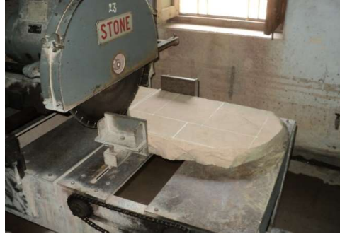
Fig. 4.2: Picture of sandstone slab cutting on disk saw
