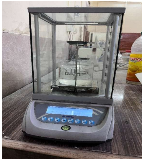
Fig. 3.6: Density measuring device based on Archimedes principle
