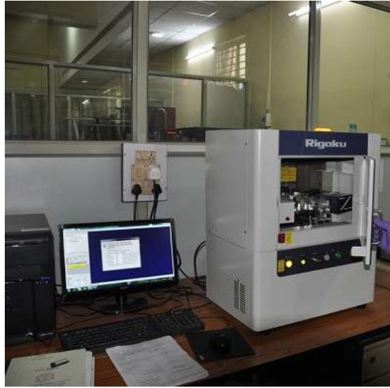
Fig. 3.5: Image of bench top X-ray diffraction instrument
