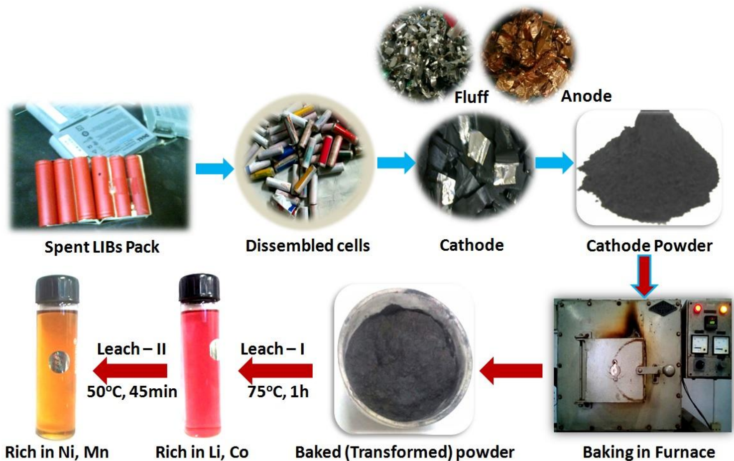
Fig. 3.47: Flowsheet of process intensification by acid baking followed by leaching to extract metallic values from LIB cathode materials
