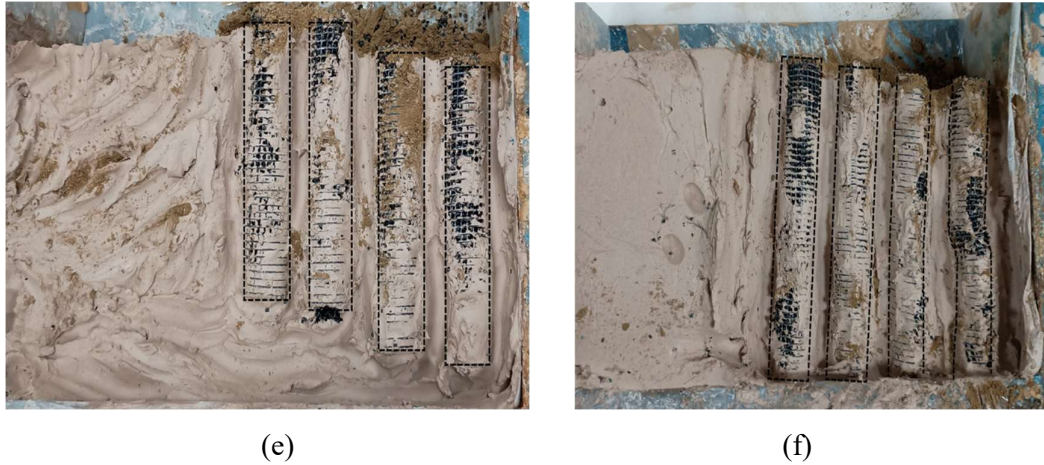
Fig. 5.12 Settlement response under cyclic loading of (a) embankment plan view, (b) embankment elevation, (c) GC FL, (d) GC EB, (e) EGC FL, (f) EGC EB.
