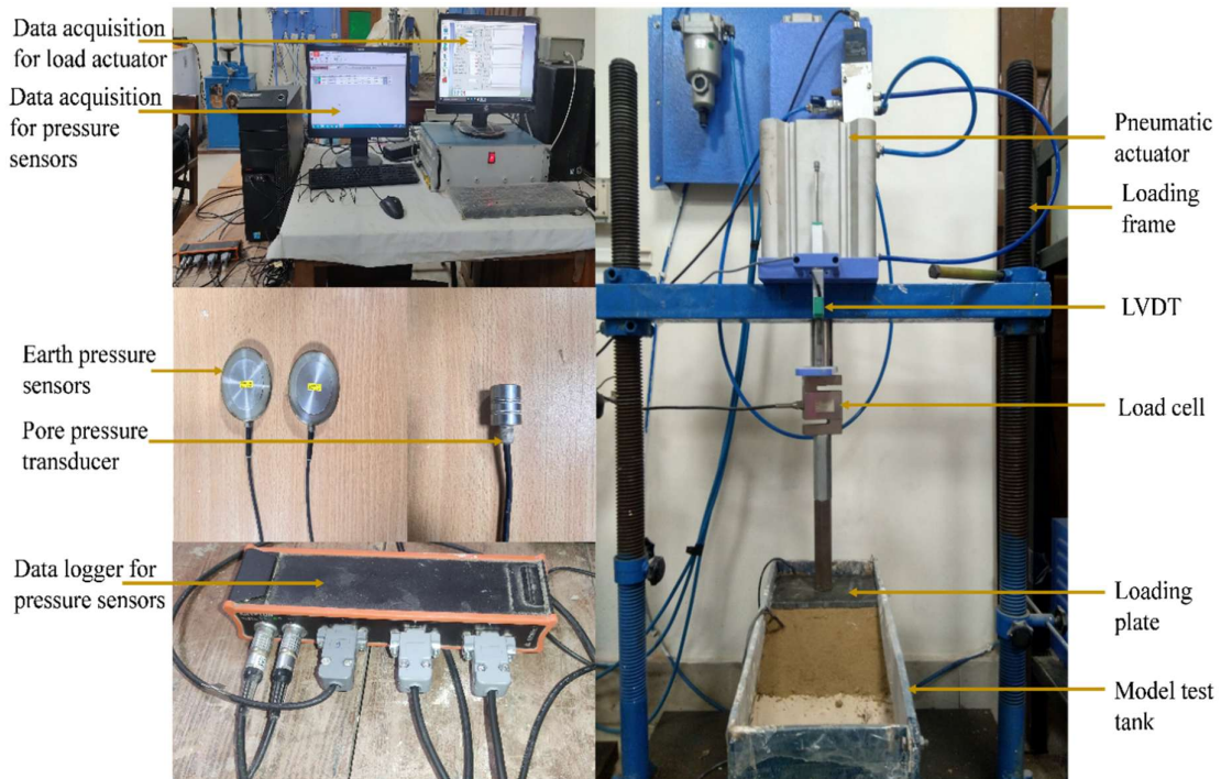
Fig. 5.1 Systematic representation of model test setup, sensors and data acquisition system.
