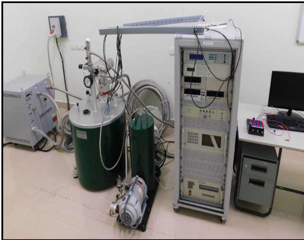
Figure 2.4 The Physical property measurement system (PPMS) set up at UGC-DAE, Kalpakkam node.
