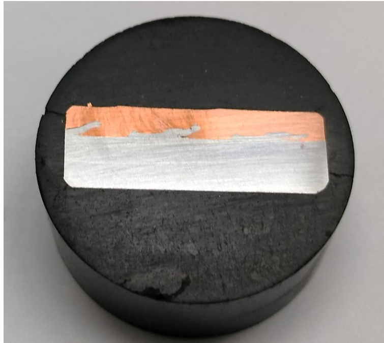
Figure 3-8 Prepared transverse cross section sample for metallography
