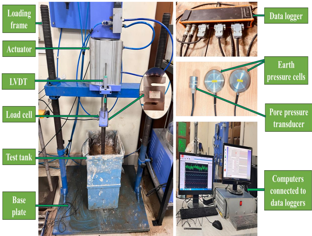
Fig. 3.11 Model test setup along with data loggers, earth pressure cells, and pore pressure transducer.
