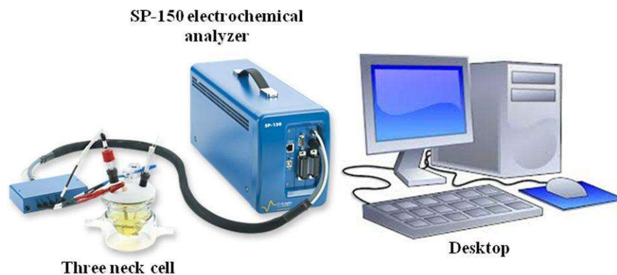
FIGURE 4.22: Schematic layout of experiment setup used for corrosion test by potentiodynamic method
