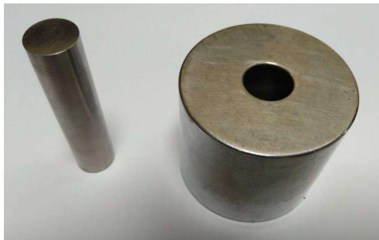
FIGURE 4.11: Die and punch assembly for preparation of pellets
