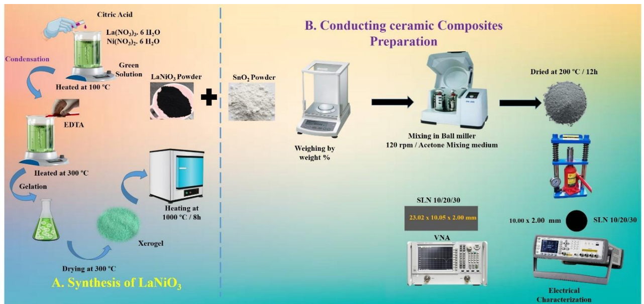
Figure 6.1 Schematic illustrating the detailed sample preparation process. (a) Synthesis of pure \text{LaNiO}_3 , (b) Steps involved in composite preparation.
