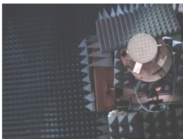
Fig. 3-85: Pattern measurement setup in test chamber of the realized 8 \times 8 -element AW-TPA array.
