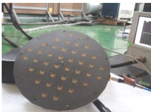
Fig. 3-84: VSWR measurement setup of the realized 8 \times 8 -element AW-TPA array.
