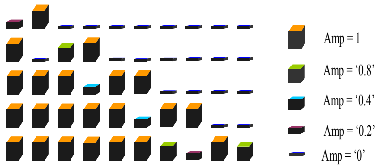
Fig. 3-49: Optimal arrangement of ‘ON’ (yellow) and ‘OFF’ (green) elements on the aperture of the proposed 10×20-element UE-TPA array.
