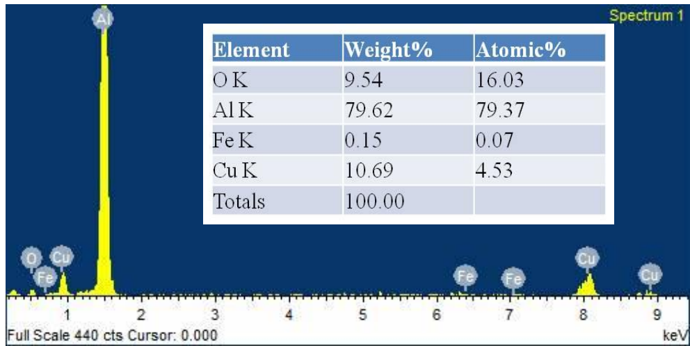
Figure 3.11: SEM micrographs and EDS analysis of 800 rpm stirring speed rheocast sample worn surfaces tested at 30 N load and 5 m/s sliding velocity at (a) lower and (b) higher magnifications.
