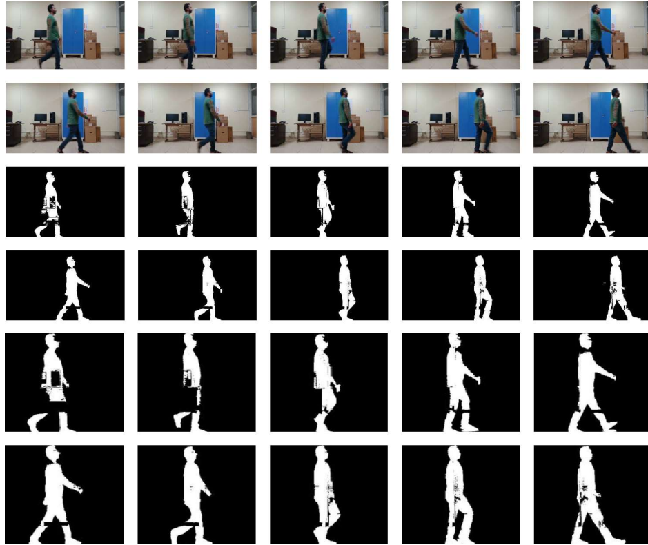
Figure 1.2: RGB to silhouette image, first two rows consist of RGB images, next two rows consist of the corresponding silhouette images before dimension normalization, and the last two rows correspond to the cropped and normalized silhouettes.
