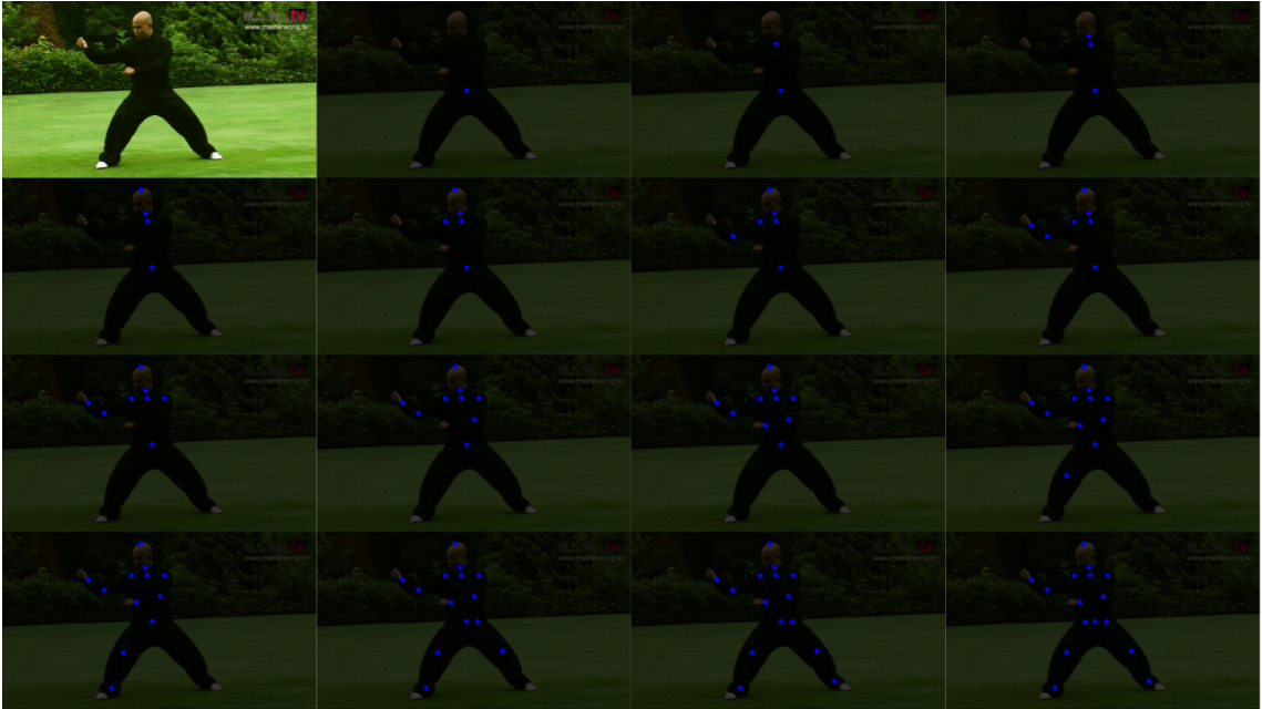
FIGURE 3.7: The visualization of heatmap for all 16 joint locations on the MPII dataset. The images from left to right and top to bottom have been added the heatmaps for pelvis, thorax, upper neck, head top, right shoulder, right elbow, right wrist, left shoulder, left elbow, left wrist, right knee, right ankle, left hip, left knee, left ankle, right hip.
